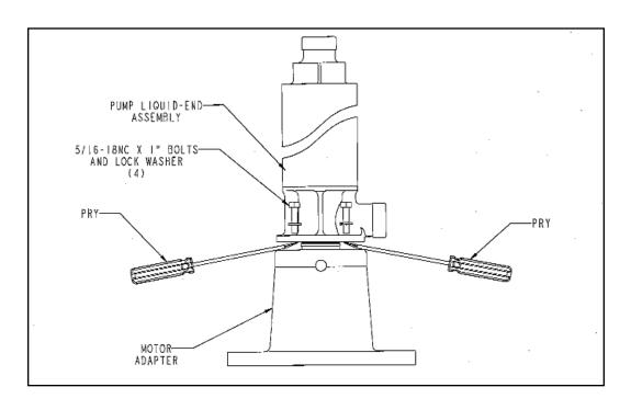
Figure 4.5 Removal of Pump Liquid-End from
